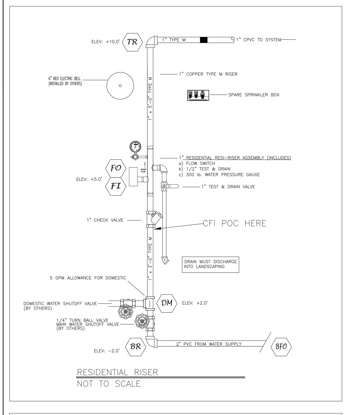
ALL RISER PIPING IS 1" RESI-RISER BRASS U.N.O. NOTE: ALL PIPING IS CENTER TO CENTER FOR SITE DETAILS SEE SHEET FP2 SIZING BASED ON CALCULATIONS. ALL NEW OVERHEAD PIPING IS 1" CPVC U.N.O.. EXTERIOR BELL TO BE MOUNTED AT LEAST SEVEN FEET ABOVE GRADE ALL UNDERGROUND FROM CITY MAIN TO BASE OF RISER MANIFOLD IS BY OTHERS
